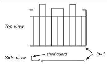
the shelf guard should be at the back pointing upwards
